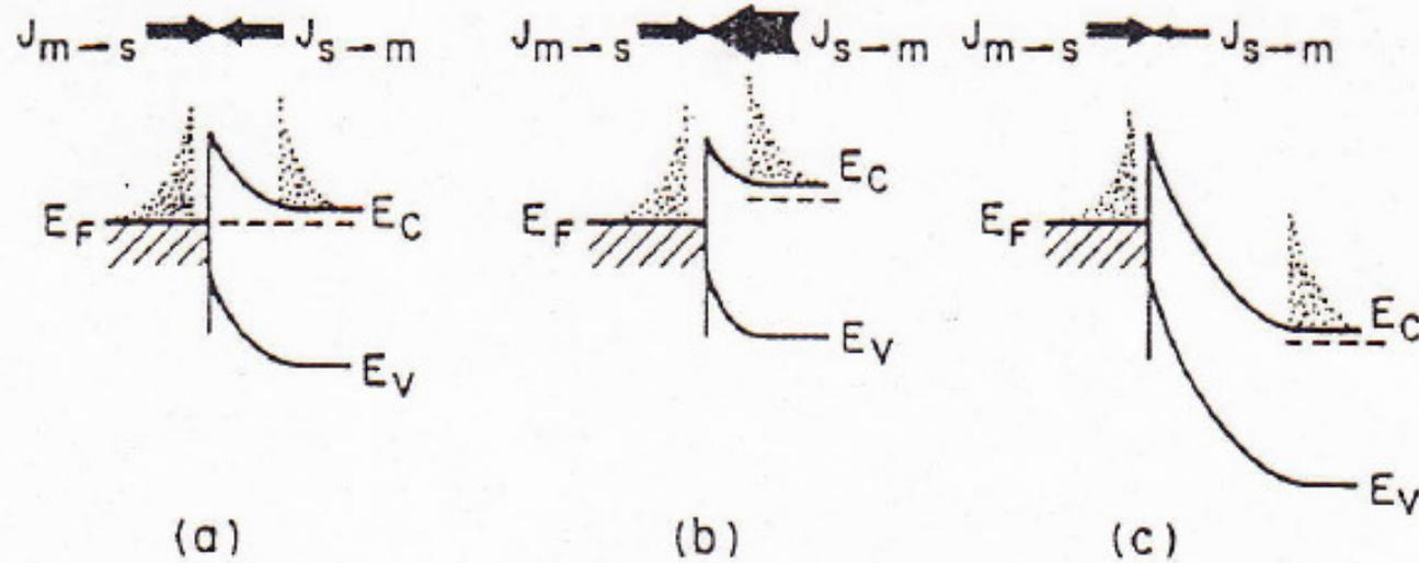
**Fig. 6** Current transport by the thermionic emission process. (a) Thermal equilibrium. (b) Forward bias. (c) Reverse bias.<sup>4</sup>
