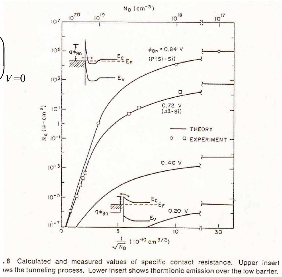
.8 Calculated and measured values of specific contact resistance. Upper insert shows the tunneling process. Lower insert shows thermionic emission over the low barrier.
