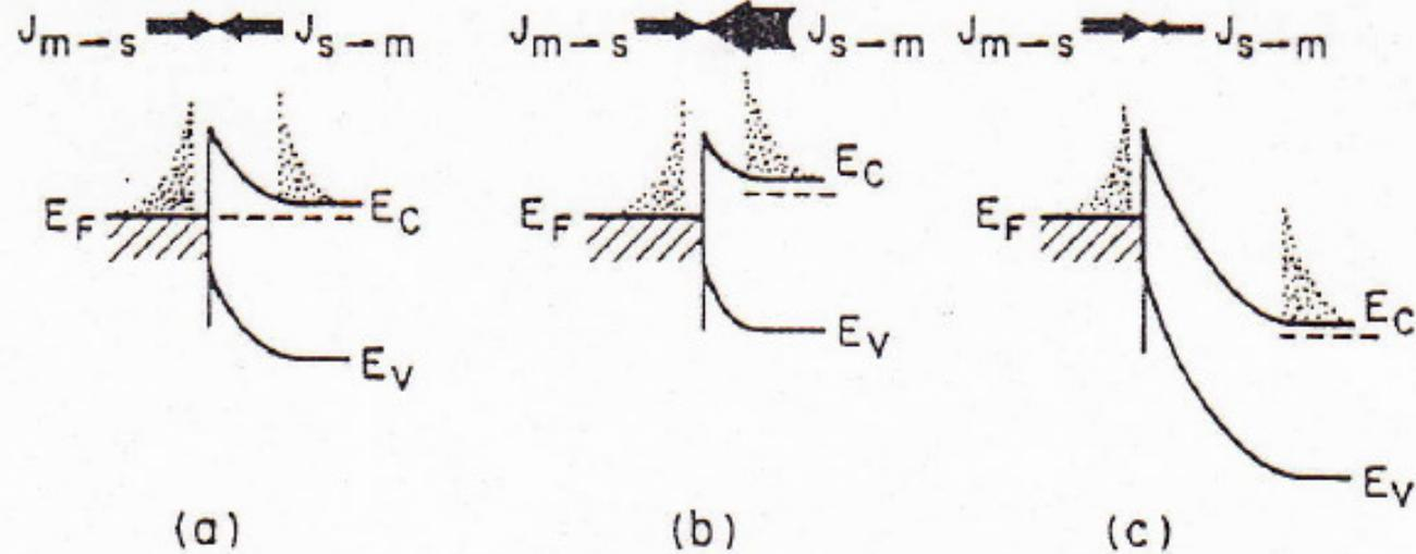
**Fig. 6** Current transport by the thermionic emission process. (a) Thermal equilibrium. (b) Forward bias. (c) Reverse bias.<sup>4</sup>
