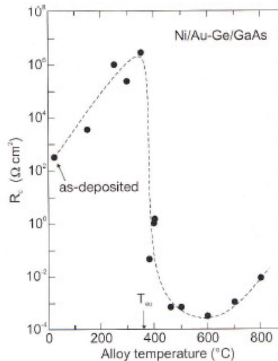
**Fig. 18.20.** Specific contact resistance for Ni/Au-Ge on n-type epitaxial GaAs for varying alloying temperatures (2 min). Arrow at  $T_{eu}$  denotes the eutectic temperature of Au-Ge. Adapted from [572]
